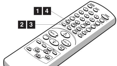
Press the SET/TR + or – button to select the AUTO CH MEMORY mode, then press the ENTER button. The TV/VCR will begin memorizing all the channels available in your area. Channel numbers will remain red until auto memorizing is complete.
